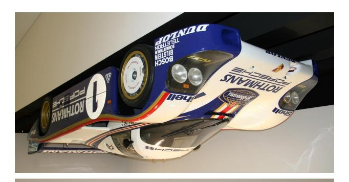
According to the theory of downforce ( $F = \varrho: 2 \cdot v^2 \cdot A \cdot c_a$ ), when this Porsche 956 reaches a speed of 321.4 km/h, it could theoretically drive on ceilings.
