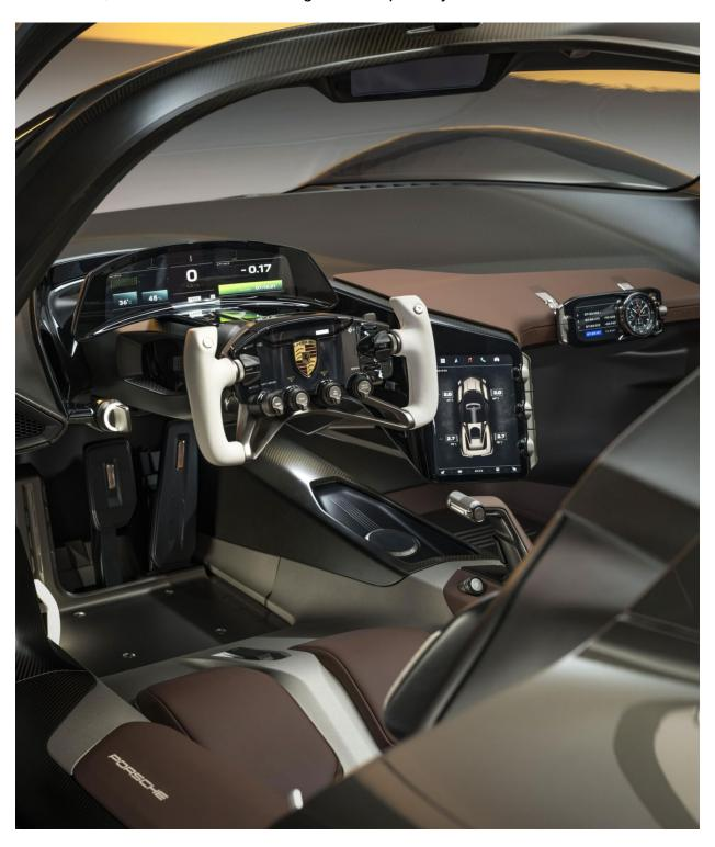
The concept uses carbon-reinforced plastic for its seats, and the six-point belts are built into the monocoque. The open-top steering wheel has controls and shift paddles at the ready. But the concept also champions the luxurious side of track-inspired driving; it features a flashily new Porsche crest that employs a bit of unspecified precious metal, a subdued gray-and-brown color scheme in the cabin, and seats that can be customized with 3D printing.
